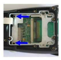
• Put the RFID Coupler HF-T2-G2-XMOD in the same alignment of the expansion connector on the WORKABOUT PRO. Apply slight pressure to snap the module into place on the hand-held.
