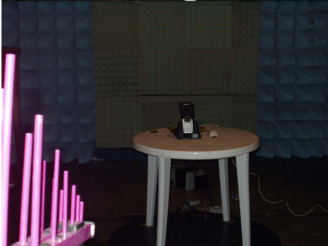
Photograph of the EUT (docked) as viewed from in front of the loop / bilog antennas, site M.
