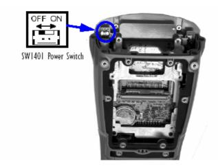
With the power shut down, you can install the RFID Module HF-T2-A1.
