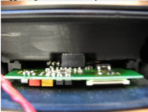
The smart card board and the reader board are plugged together with a 8-ways SIL connector
