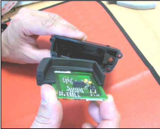
Put silicon between the rubber and the reader board ....
