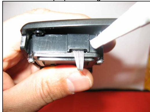
Put silicon in the MSO cable window to ensure proper sealing
