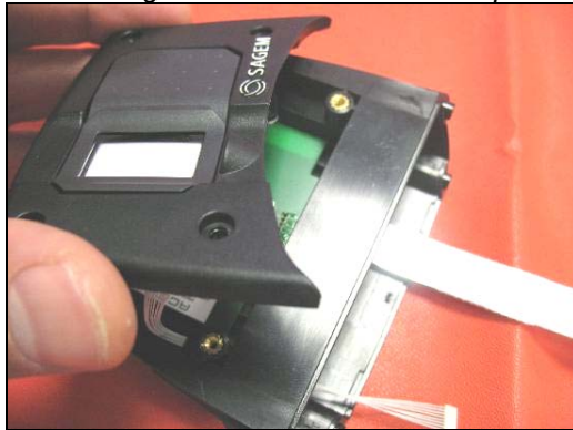
Pass the 8 way connector of the fingerprint unit through the window of the endcap
