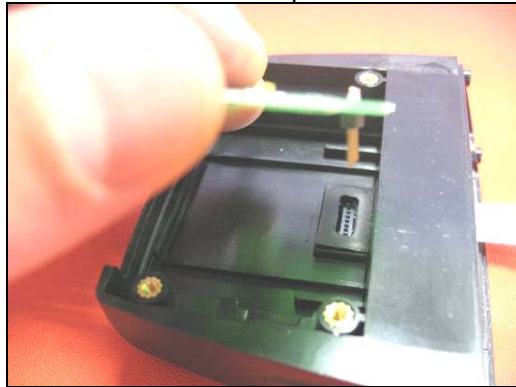
Pass the 8 way connector of the fingerprint unit through the window of the endcap
