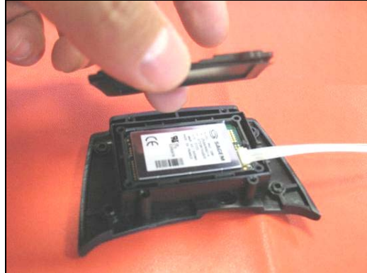
Put silicon in the MSO cable window to ensure proper sealing
