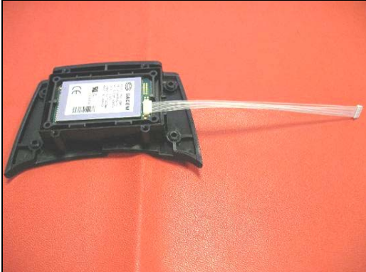
Connect the MSO cable to the MSO sensor
