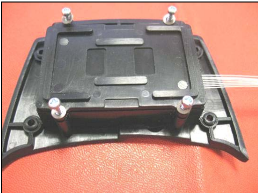
Screw the 4 self tapping screws with their washer
