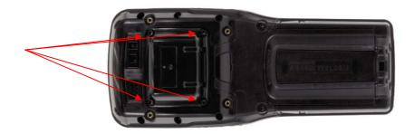
You can now install the RFID Module HF-AM1-OMNII
