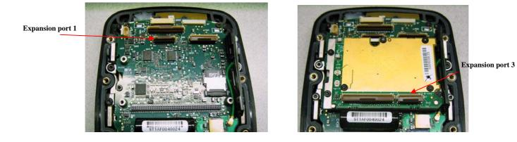
1. Expansion port 1: Connect the Flex cable to the main logic board as shown hereafter:
