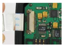
• The RFID module HF-AM1-OMNII can be plugged on the OMNII using either expansion port 1 or expansion port 3. (GPS option)
