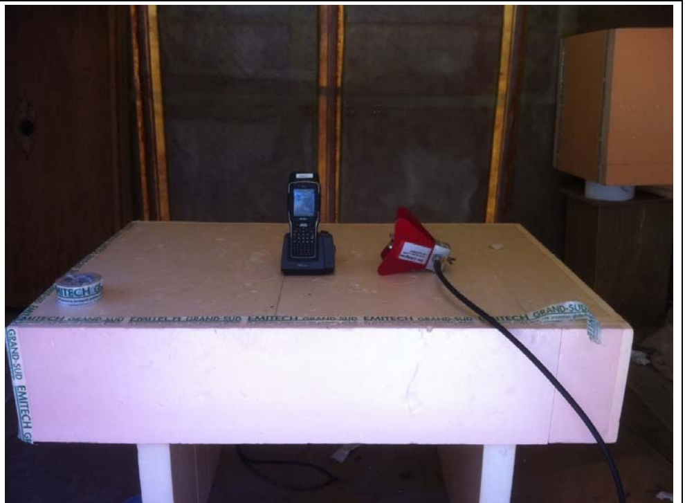
Radiated electric field emission on OATS
