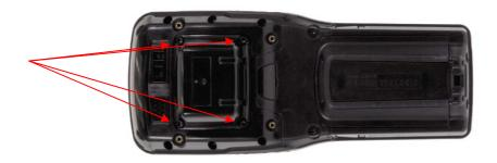
You can now install the RFID Module HF-AM1-OMNII
