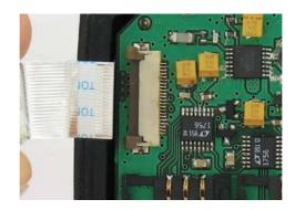
• The RFID module HF-AM1-OMNII can be plugged on the OMNII using either expansion port 1 or expansion port 3. (GPS option)
