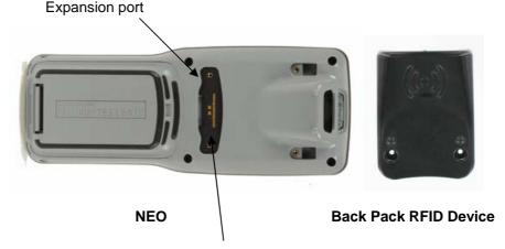
**Important:** Remove the expansion port plastic part before a back pack RFID module is being installed.
