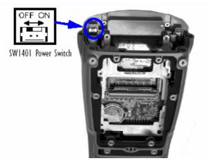
With the power shut down, you can install the RFID Module HF-AM1-A2.
