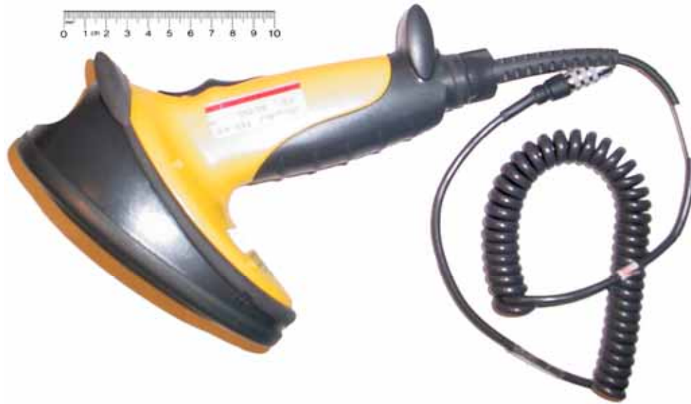
< PSC Decoded laser scanner (M/N: POWERSCAN) >
