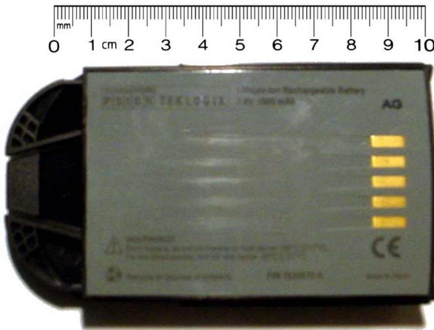
< Lithium-Ion rechargeable battery (P/N: 1030070 A-001, 7.4 V, 1800 mAh) >
