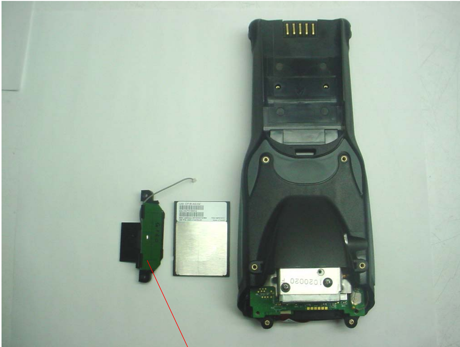
Psion Teklogix Antenna, Model: 1020096-100, Gain 0 dBi
