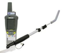
• Hook the mounting plate of the AEA120 into the bottom of the Workabout PRO. Fit both together, so that the screw holes match.
