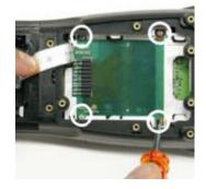
• Stick the RFID Module LF-AIR200-G2-XMOD to the WORKABOUT PRO, as shown.
