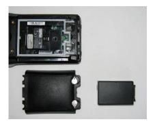
• Slide the switch to position OFF to shut off internal battery power.
