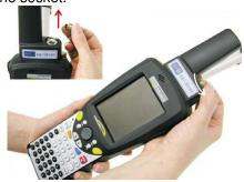
• Put the Binder plug of the telescope antenna in the socket of the RFID Module LF-AIR200-G2-XMOD.
