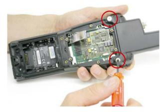
• Fix the four screws on the top of the end cap.
