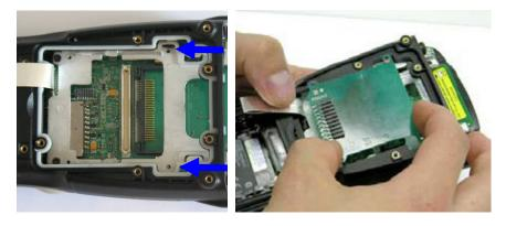
• Put the adapter board in the same alignment of the expansion connector on the WORKABOUT PRO. Apply slight pressure to snap the module into place on the hand-held.
