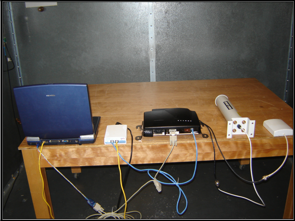
Photograph 10: Conducted Line Emissions Testing; Powered Over Ethernet - Rear View
