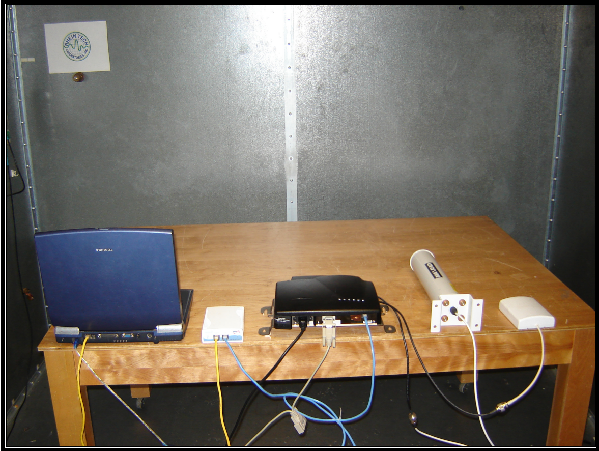
Photograph 8: Conducted Line Emissions Testing; AC Powered - Rear View
