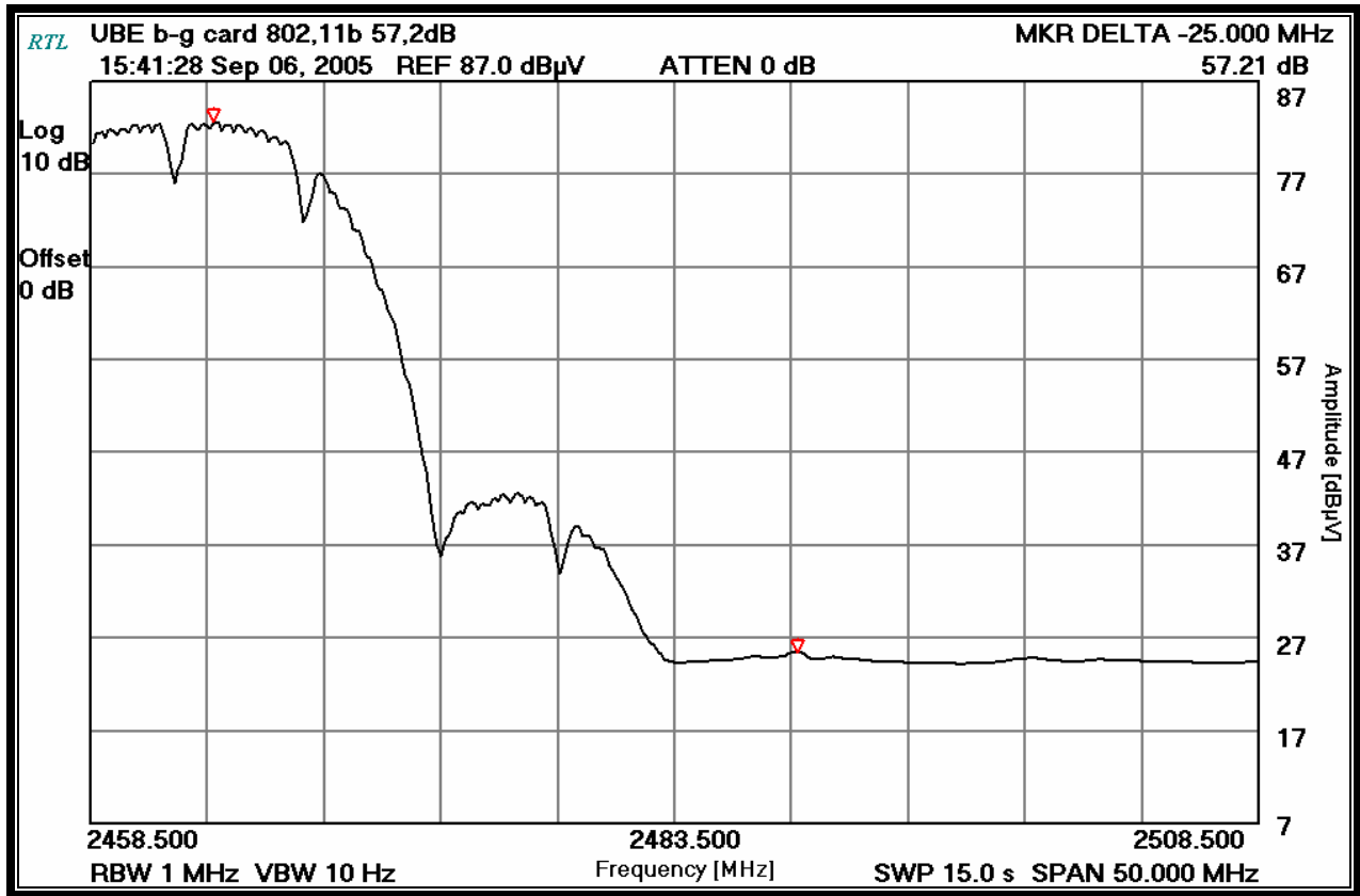
Plot 3-2: Upper Band Edge: Average Measurement Channel 11 (TX Frequency: 2462 MHz – 1 Mbps) Omni Antenna
