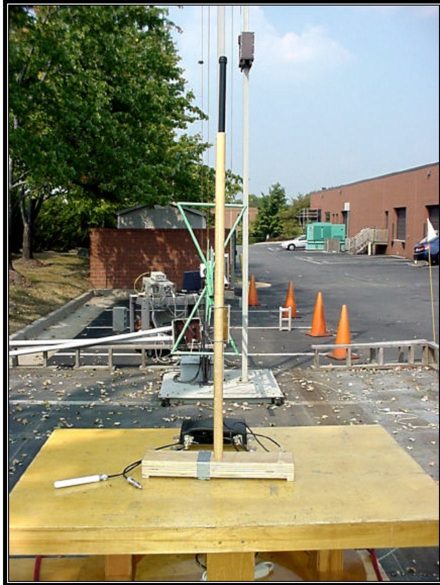
Photograph 5: Radiated Testing – 12 dBi Collinear Omni Rear View
