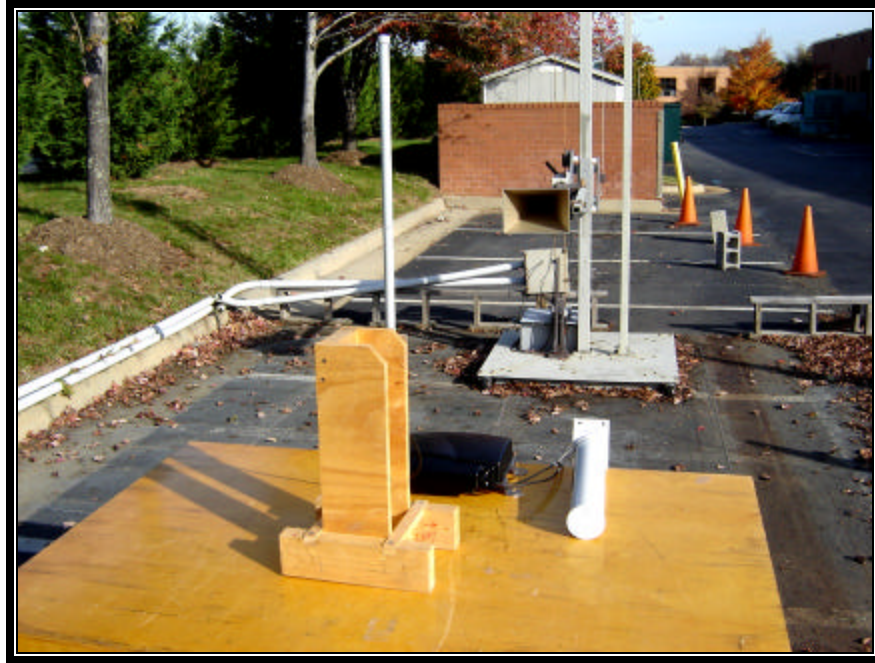
Photograph 11: Radiated Testing – 12 dBi Pacific Collinear Omni Rear View
