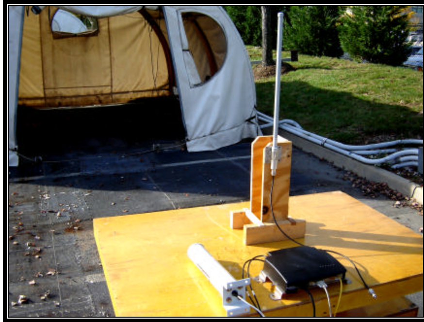
Photograph 10: Radiated Testing – 12 dBi Pacific Collinear Omni Front View
