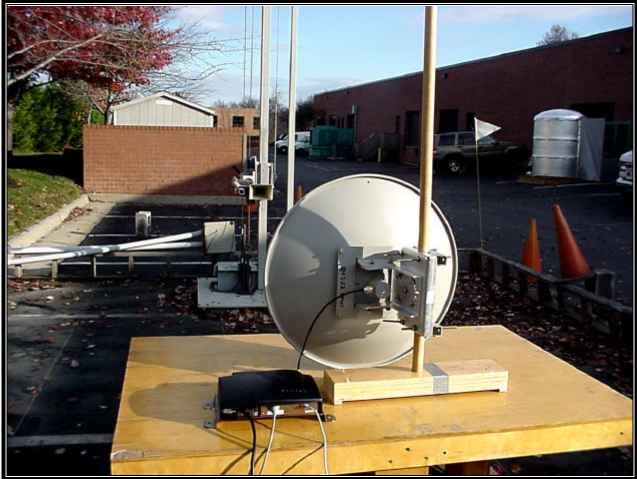
Photograph 9: Radiated Testing – 28 dBi Gabriel Dish Rear View
