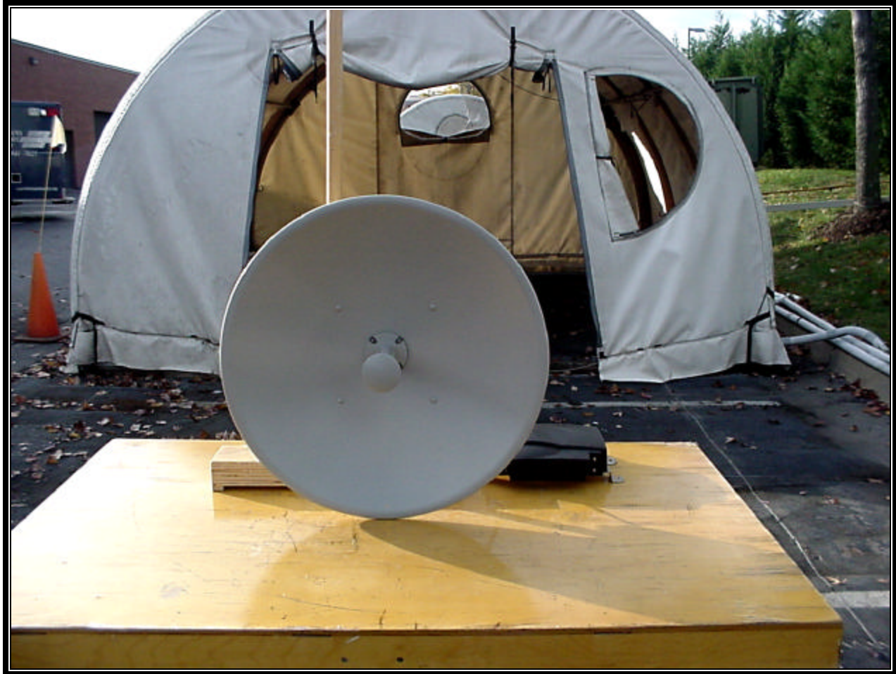
Photograph 8: Radiated Testing – 28 dBi Gabriel Dish Front View
