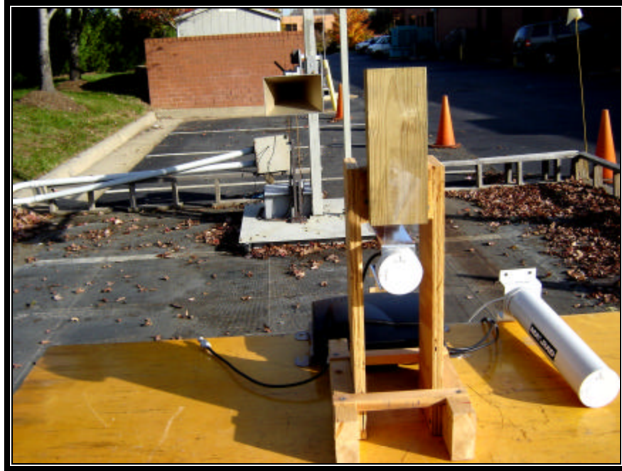
Photograph 14: Radiated Testing – 10 dBi MaxRad Panel Front View
