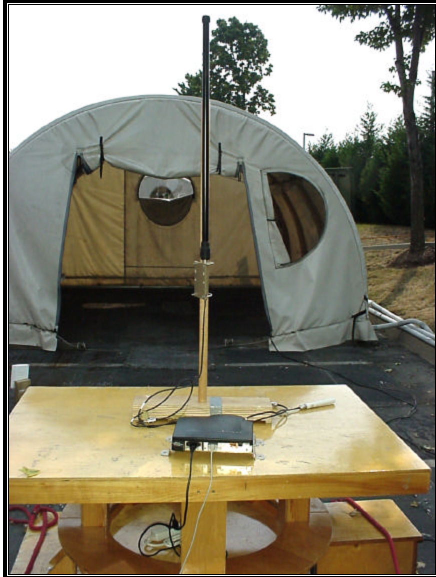
Photograph 4: Radiated Testing – 12 dBi Collinear Omni Front View
