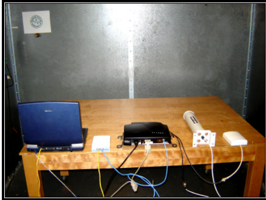
Photograph 19: Conducted Line Emissions Testing; AC Powered - Rear View
