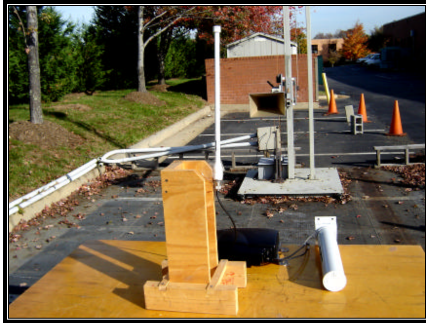
Photograph 12: Radiated Testing – 10 dBi MaxRad Omni Front View
