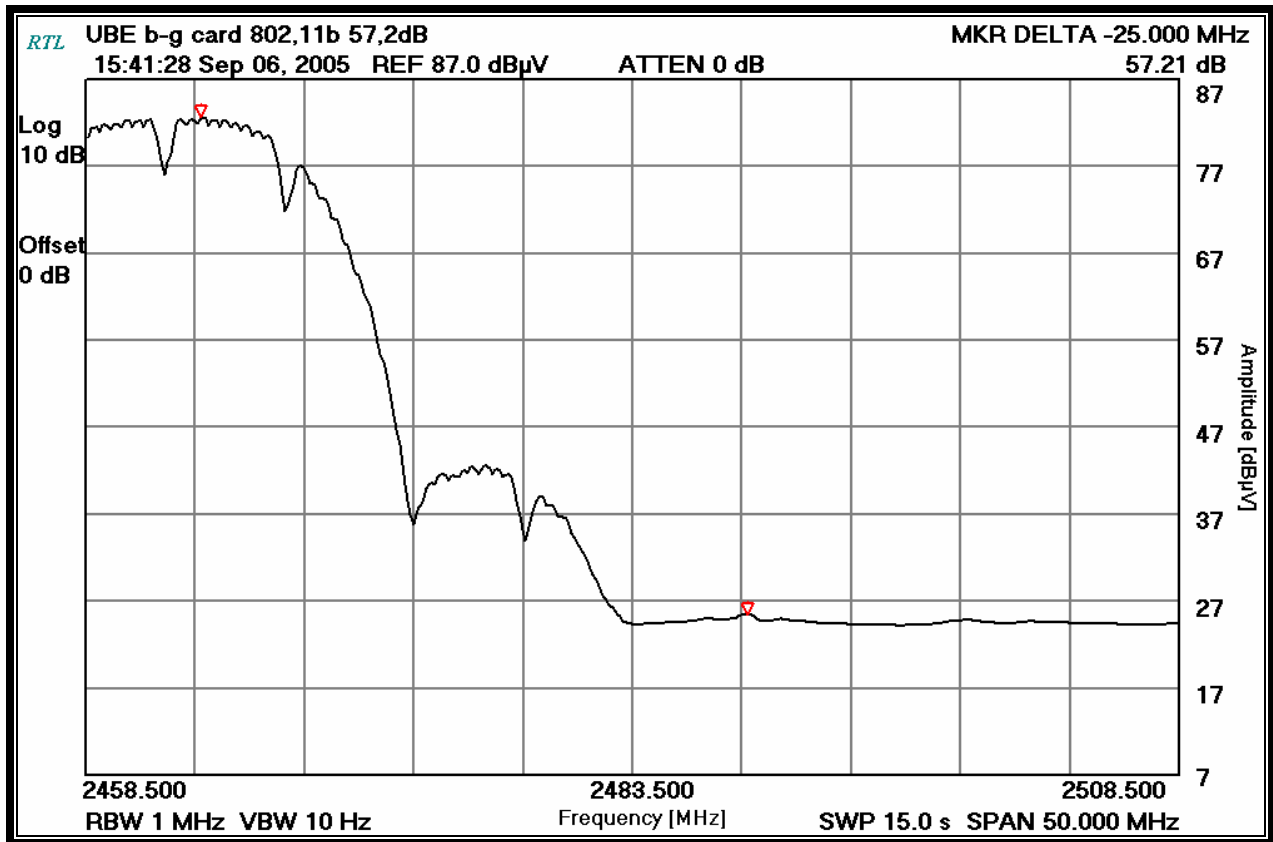
Plot 4-2: Upper Band Edge: Average Measurement Channel 11 (TX Frequency: 2462 MHz – 1 Mbps) Omni Antenna
