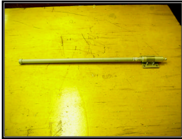
Photograph 47: Pacific OD58-12 12 dBi Collinear Omni Antenna
