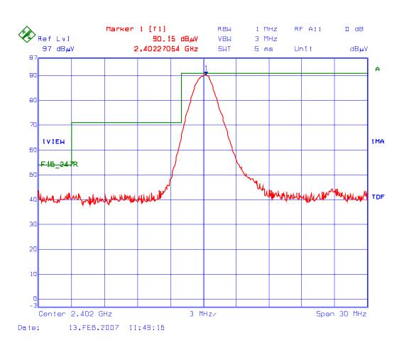
Plot 5.7.5.1.1: Band-Edge Radiated Emissions @ 3 meters Vertical Polarization, Low End of Frequency Band, Single Frequency Mode
