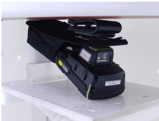
Back with Holster(ST6091), Test Separation 0 mm
