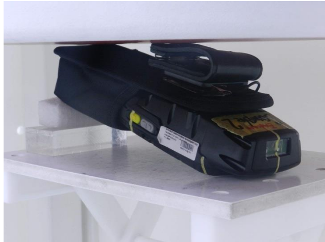
Front with Holster(ST6091), Test Separation 0 mm Back with Holster(ST6091), Test Separation 0 mm
