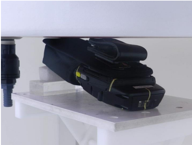
Front with Holster(ST6091), Test Separation 0 mm Back with Holster(ST6091), Test Separation 0 mm
