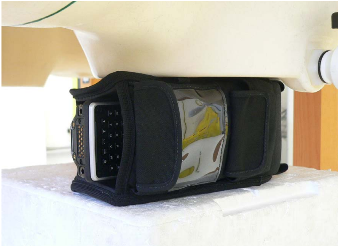
Fig. 45: Body worn configuration, position 1 with holster, left side of display in direct contact against the flat phantom.
