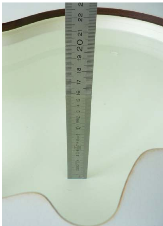
Fig. 49: Liquid depth for IEEE 802.11 b/g/n Head measurements
