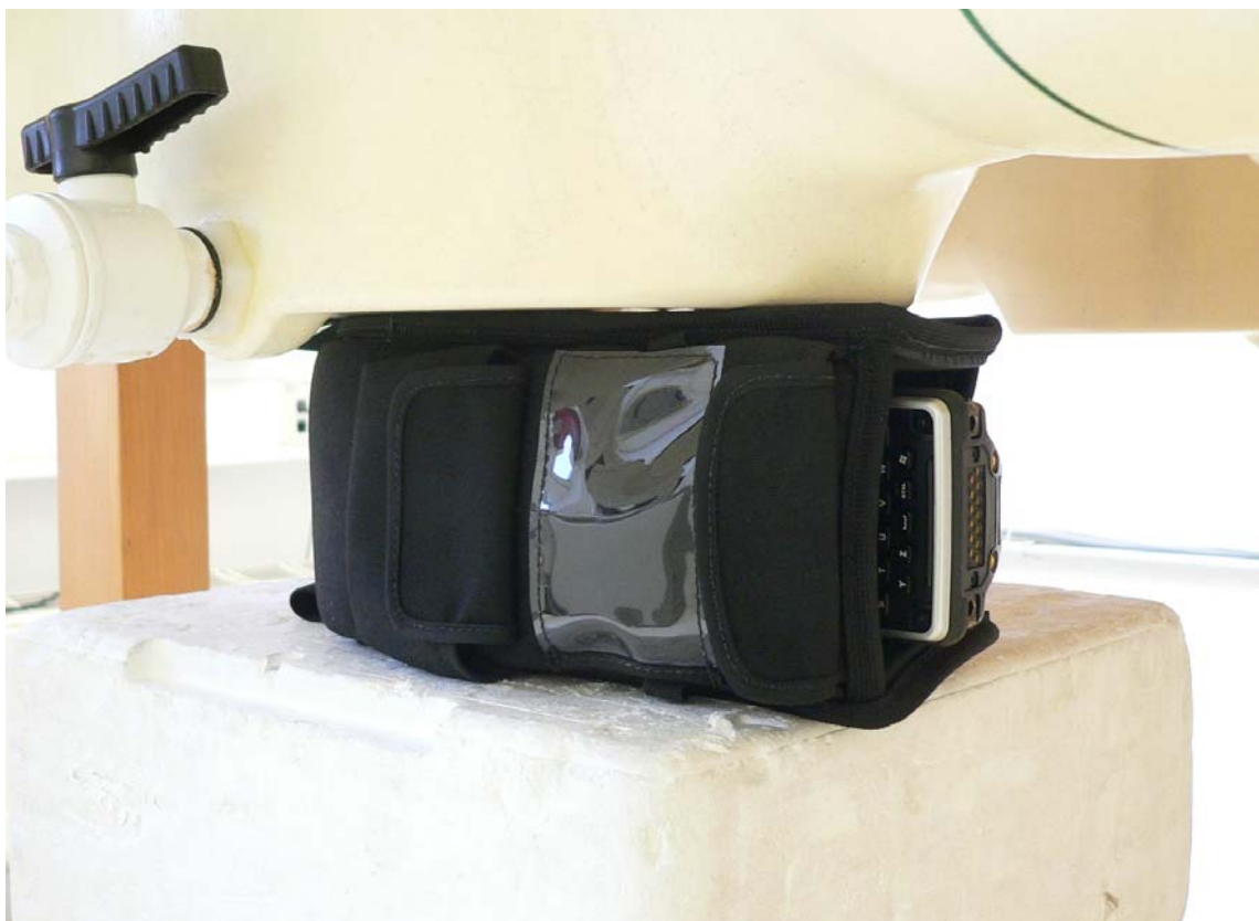
Fig. 46: Body worn configuration, position 2 with holster, right side of display in direct contact against the flat phantom.
