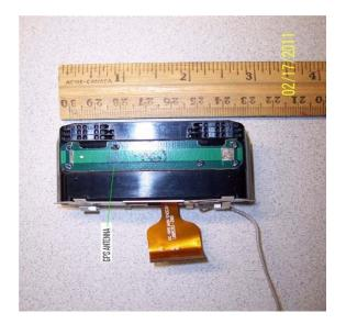
This view of the PC II change shows the same end cap but this time with the extra antennas for the 7545MBWP radio.
