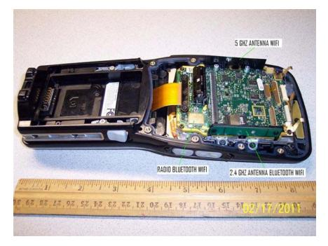
This is the original certification showing the Main Logic Board (MLB), BT/WIFI radio and antennas.
