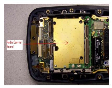
For the PC II we added the shielded 7545MBWP radio on top of the RCB, as shown here.
