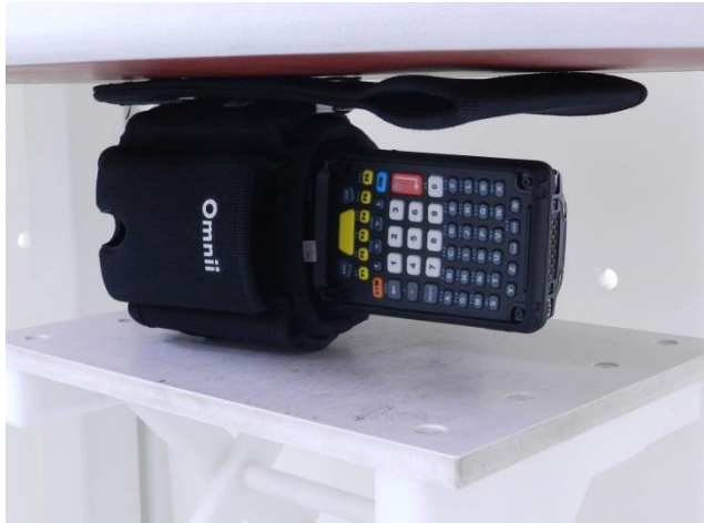
Right side with Holster(ST6056), Test Separation 0 cm
