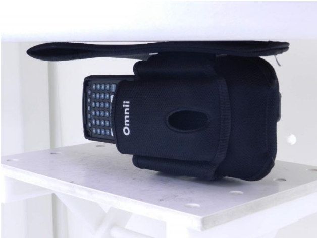
Left side with Holster(ST6056), Test Separation 0 cm
