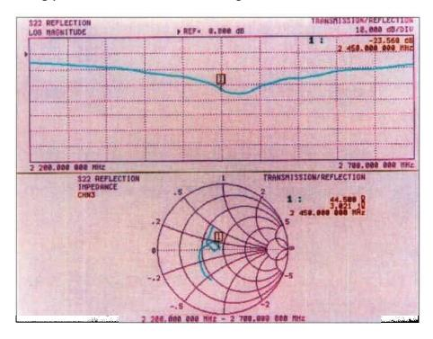
Dipole impedance at 2450 MHz Re{Z} = 44.5  $\Omega$  Im{Z} = 3.0  $\Omega$
