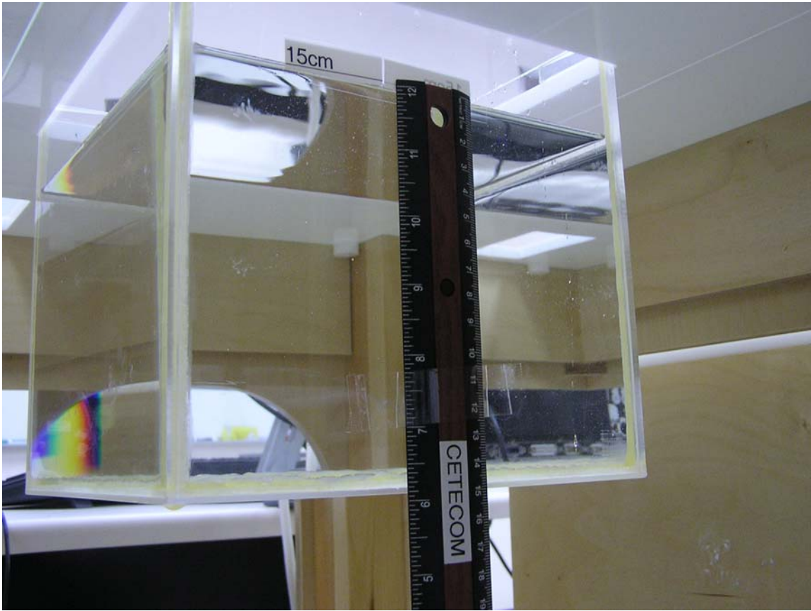
Photo 2. Photo to demonstrate 15 cm Z-axis flat phantom
