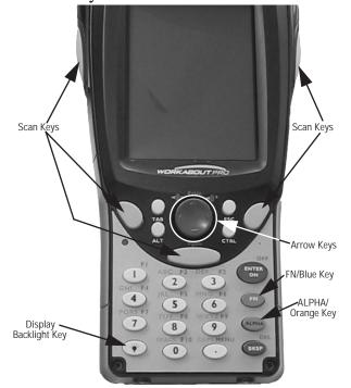
The keyboard is equipped with a set of standard keys along with a <ALPHA/ORANGE> and a <FN/BLUE> modifier key to provide access to additional keys and system functions. These extra keys are colour coded in *orange* and *blue* print above the standard keys.
