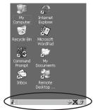
A taskbar at the bottom of the screen displays icons through which you can view the security level and battery capacity. A unit equipped with a Bluetooth radio displays the appropriate icon in the taskbar. A hand-held attached to a charger, cradle or docking station displays the associated icon, and so on.
