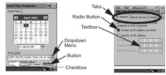
Note: Tap the stylus on a dialogue box element to select or deselect it, display a dropdown menu and so on. To use the keyboard, refer to "Navigating Using The Keyboard" on page 24.
