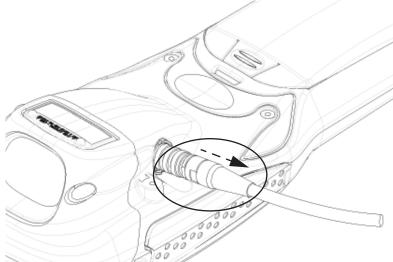
Figure 3.9 Disconnecting The Tether Cable
