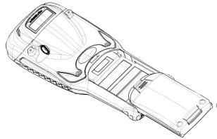
Figure 2.4 Installing The Battery
