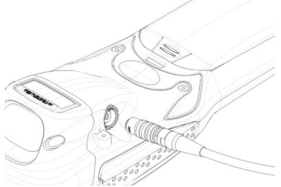
Figure 3.8 Attaching The Cable To The Tether Port
