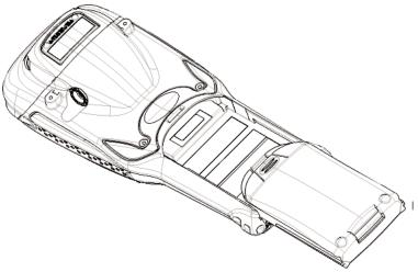
Figure 3.3 Installing The Battery Pack
