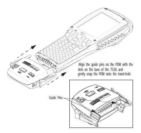
Figure 7.1 Attaching The PDM To The Base Of The 7530
