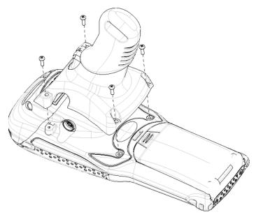
Figure 2.3 Attaching The Pistol Grip
