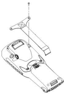
Figure 2.1 Attaching The Hand Strap
