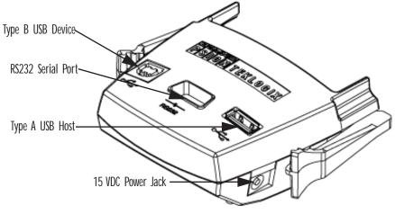
Figure 7.2 PDM Ports And Connectors
