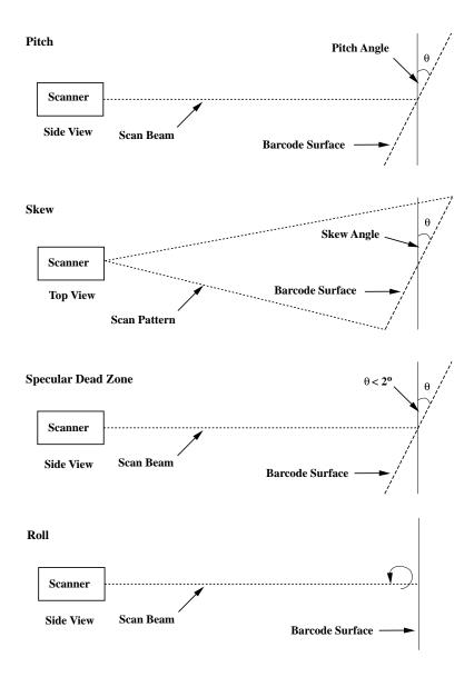
Figure 8.1 Pitch, Skew And Specular Dead Zone
