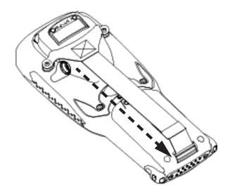
Figure 2.2 Hooking The Hand Strap To The 7530
