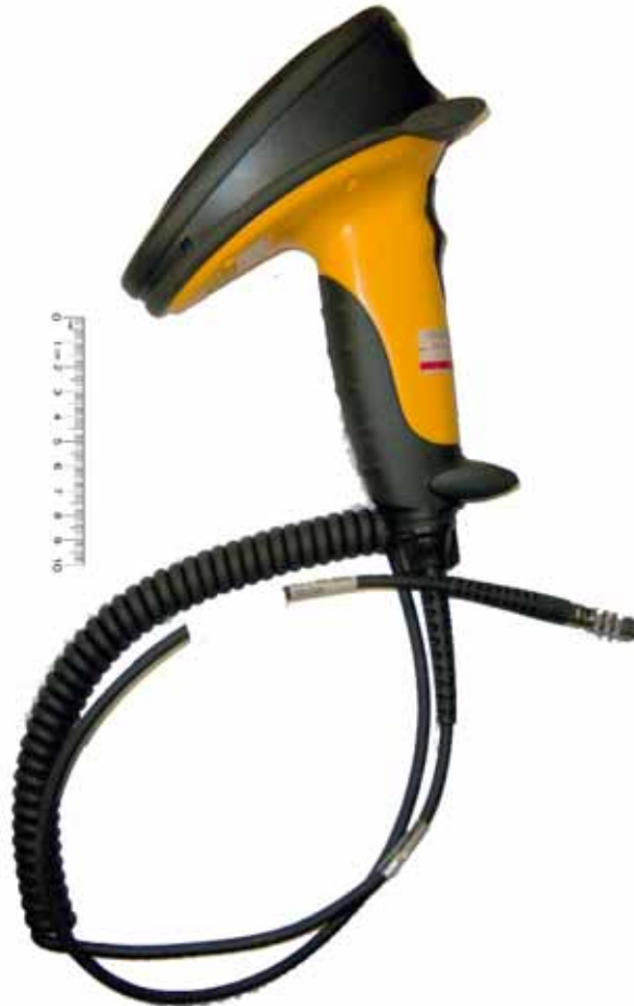
< Scanner – decoded PDF 417, 2D (Symbol M/N: P304IMG-I000) >
