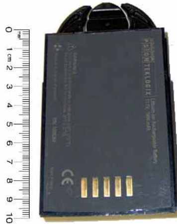
< Lithium-Ion rechargeable battery (M/N: F41001658, 11.1V, 1900mAh) >
