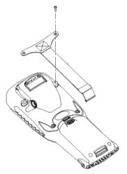
Stretch the handstrap toward the base of the 7530 G2, and hook the bottom of the handstrap into the slot near the base of the battery pack.
