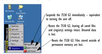
Note: The Shutdown menu varies depending on the security level chosen. At 'Supervisor' security level, a sub-menu like the one in the sample screen is displayed. At 'User' security level, choosing 'Suspend' causes the computer to shut down immediately. A sub-menu is not available.
