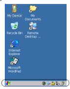
The 7530 G2 is equipped with a taskbar at the bottom of the screen. It displays icons through which you can view the security level, battery capacity and radio signal quality of your unit. A 7530 G2 attached to a charger, cradle, docking station or PDM displays the associated icon
