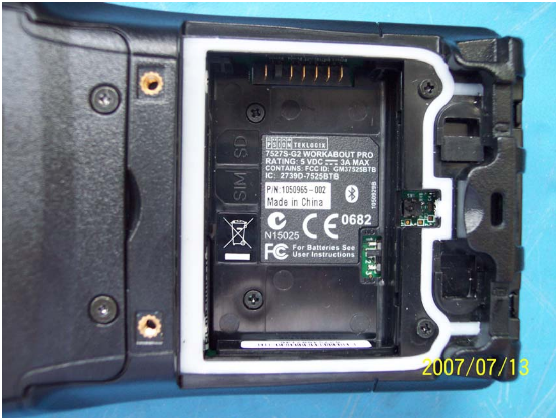
7527S – G2 Back view, Battery compartment
