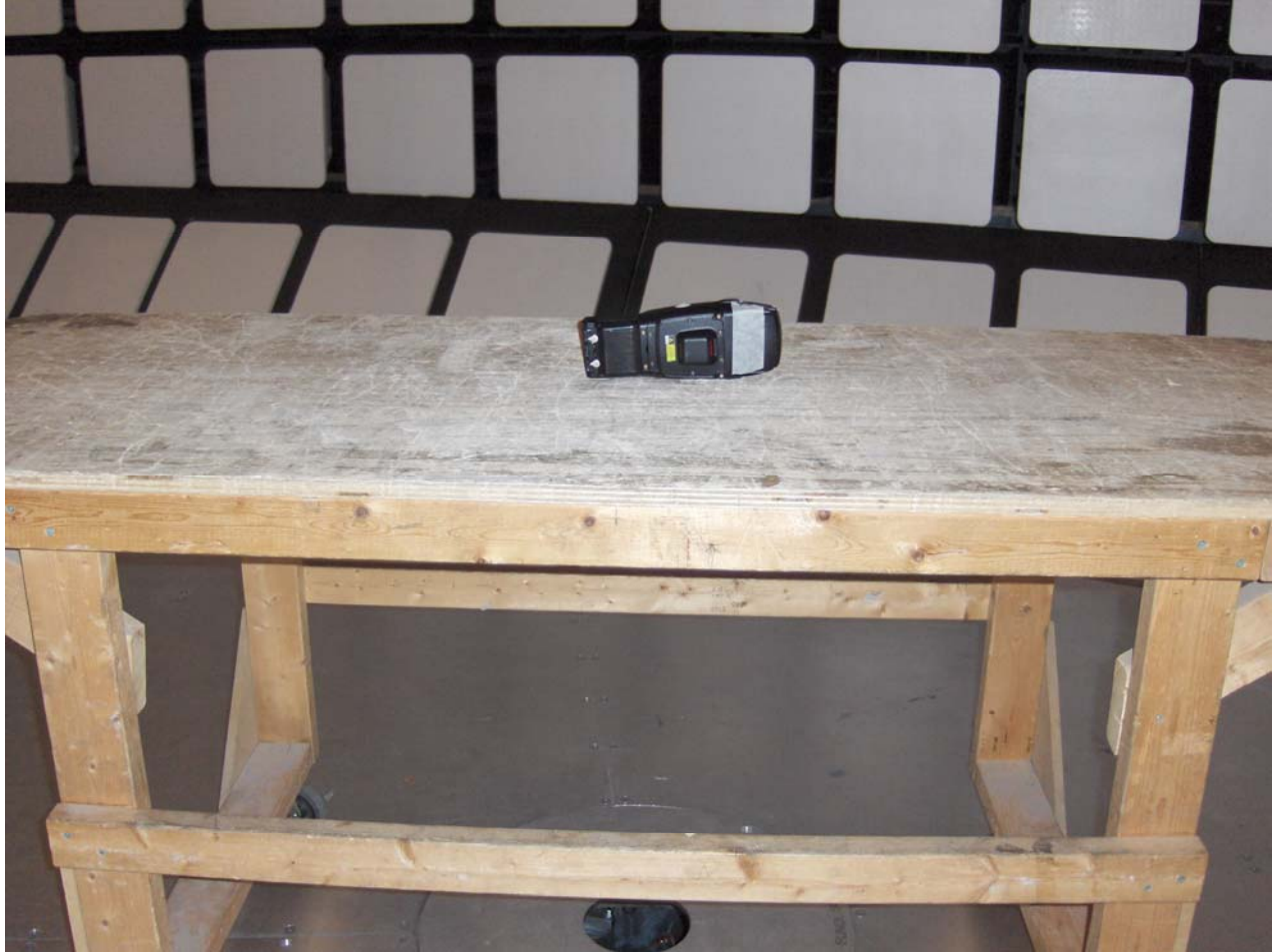
Photo #2: Radiated Emissions at 3 m Distance (Orthogonal Position #2)
