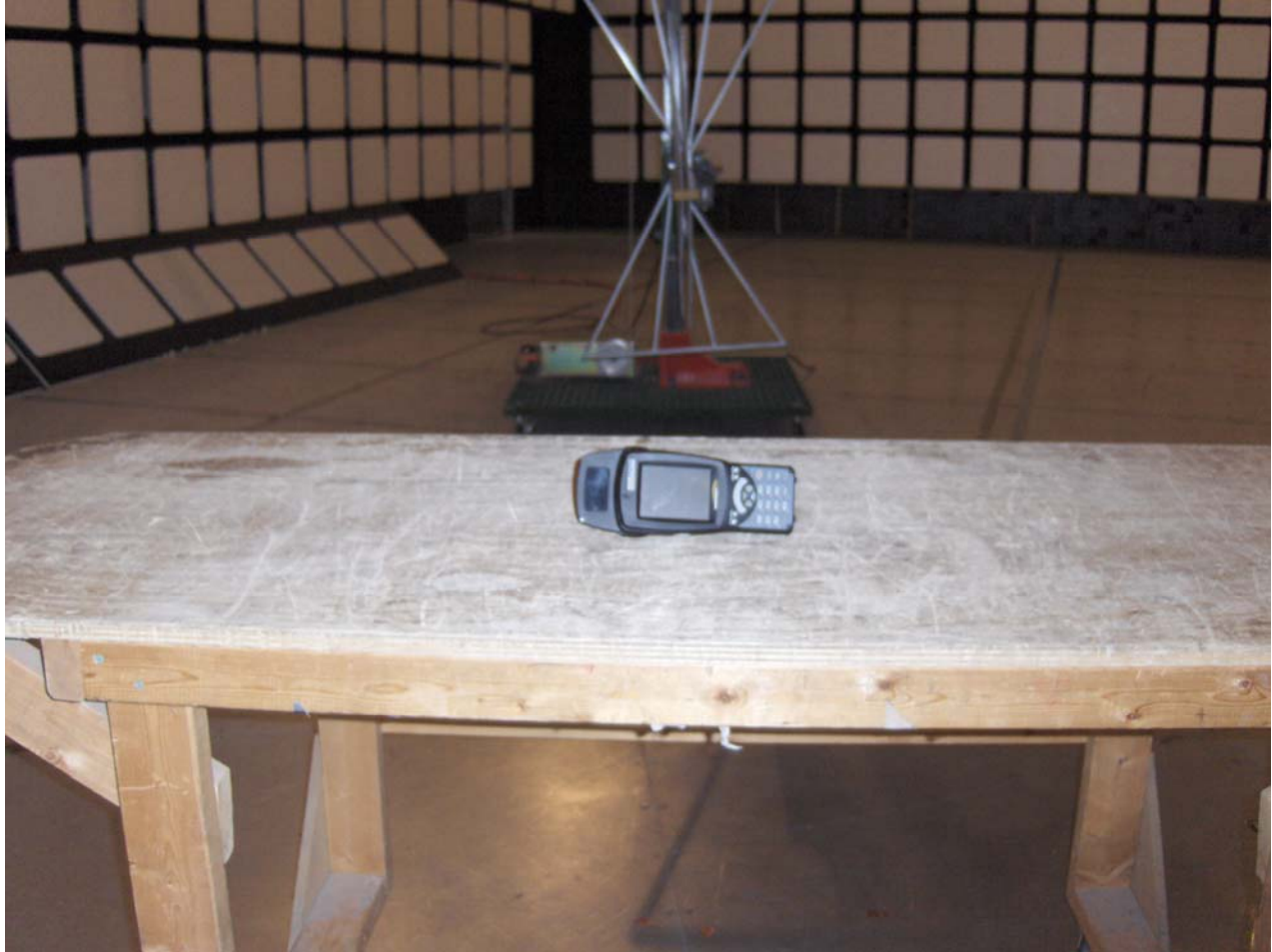
Photo #1: Radiated Emissions at 3 m Distance (Orthogonal Position #1)
