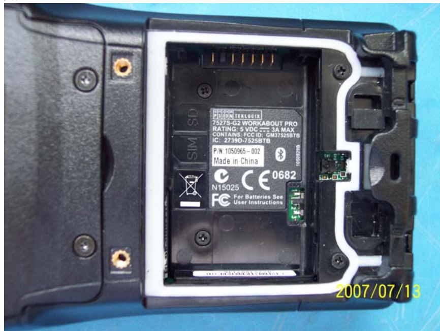
7527S – G2 Back view, Battery compartment
