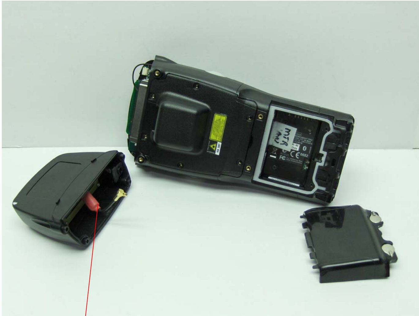
WJ RFID Radio antenna location
