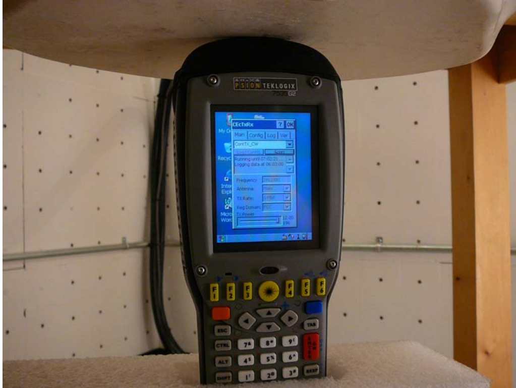
EUT Top Side touching to the flat phantom
