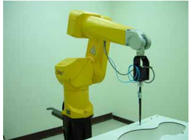
Fig. 5.2 Probe setup on robot
