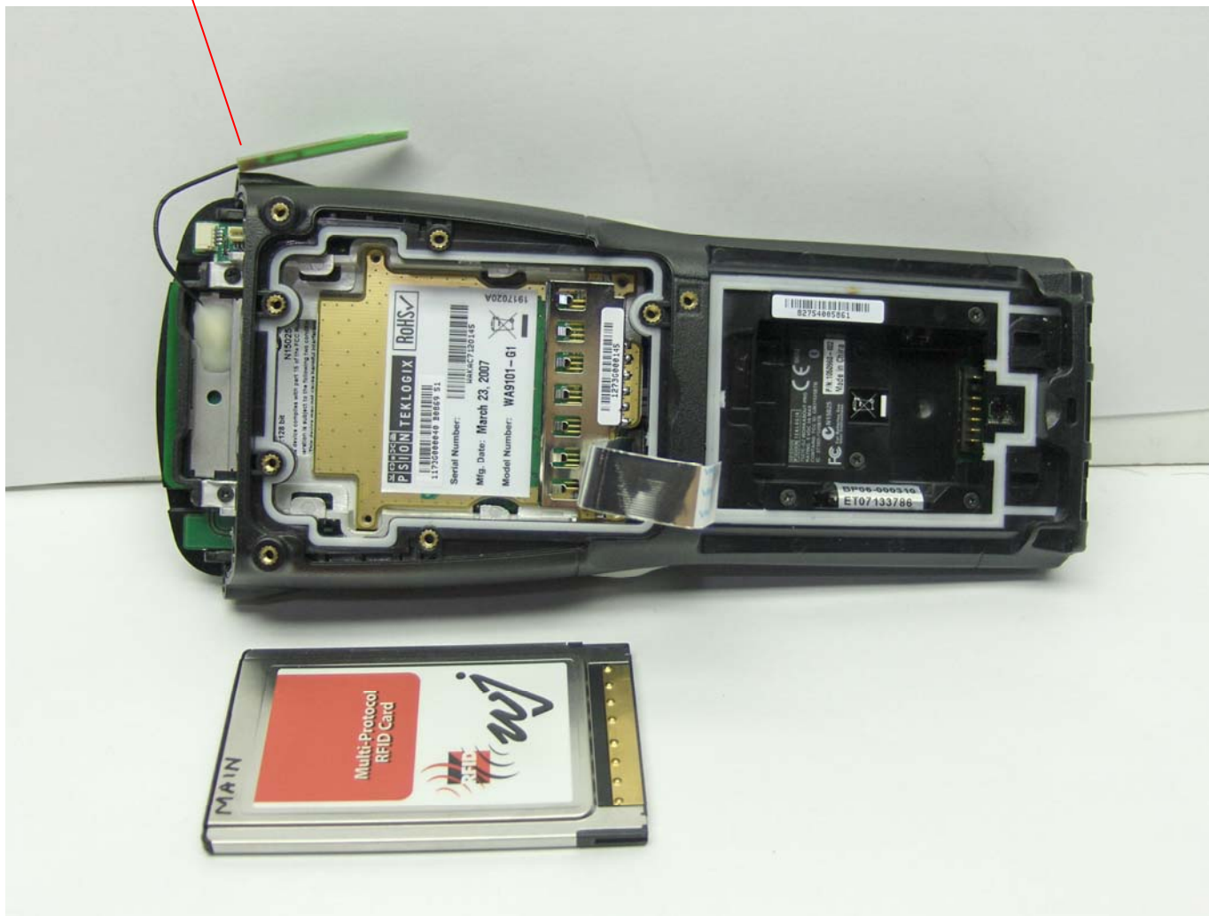
Psion Teklogix, Inc. WORKABOUT PRO G2 HANDHELD COMPUTER, Model No.: 7527C with WJ MPR6000 Radio Module (FCC ID: NTTWJMPR6XXX) FCC ID: GM37527CBTRA2041M
