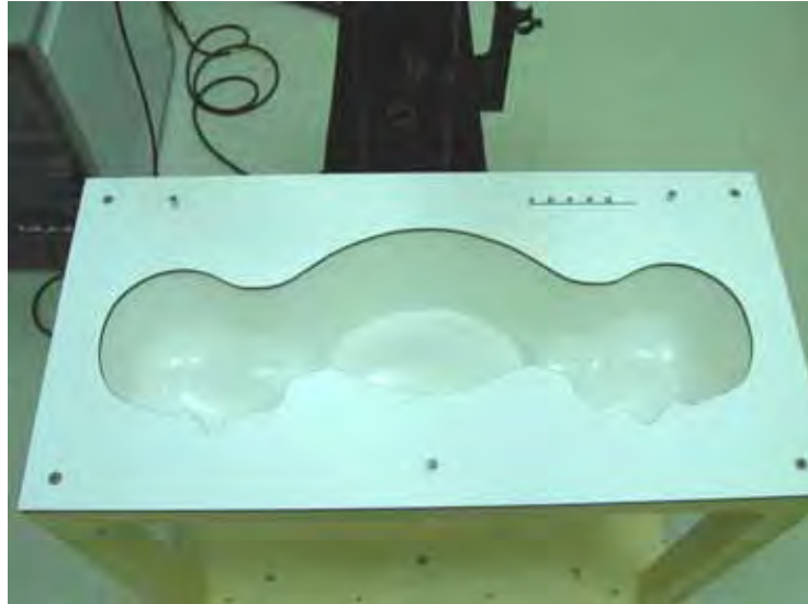
Fig. 5.3 Top view of twin phantom
