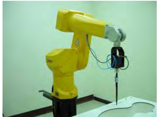
Fig. 5.2 Probe setup on robot
