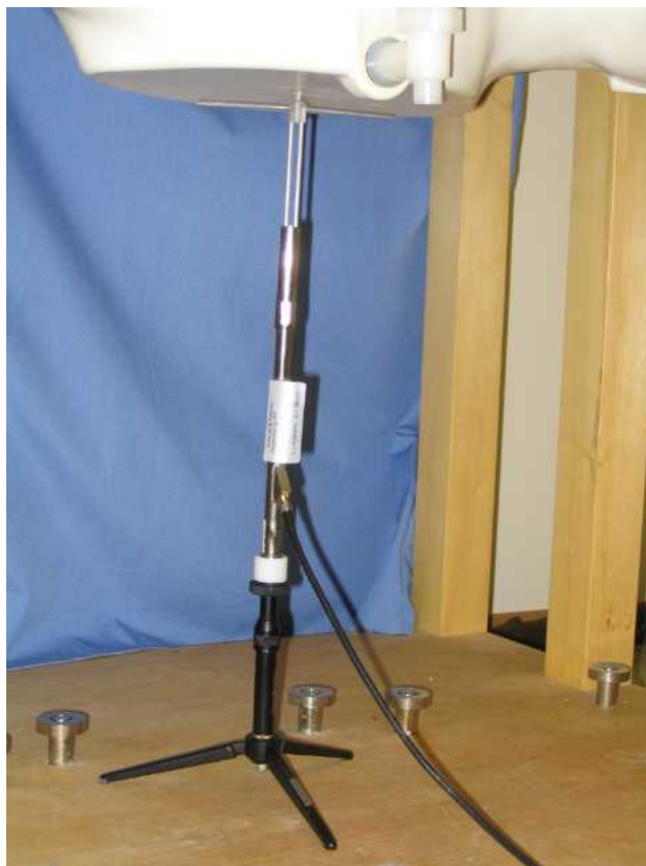
Figure 2: Photograph of System Verification (900MHz Dipole Positioned at Flat Phantom) 2
