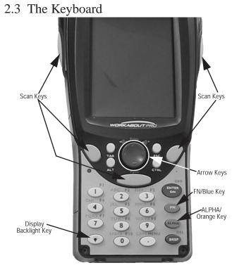
The keyboard is equipped with a set of standard keys along with a <ALPHA/ORANGE> and a <FN/BLUE> modifier key to provide access to additional keys and system functions. These extra keys are colour coded in *orange* and *blue* print above the standard keys.
