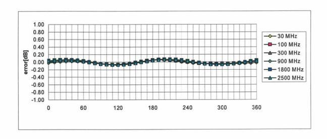
Axial Isotropy Error < ± 0.2 dB
