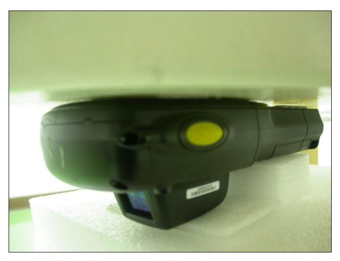
The front of the EUT to the flat phantom distance 0 mm
