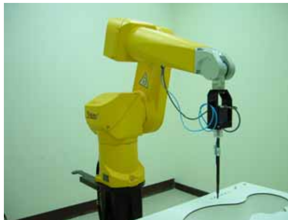
Fig. 5.2 Probe setup on robot
