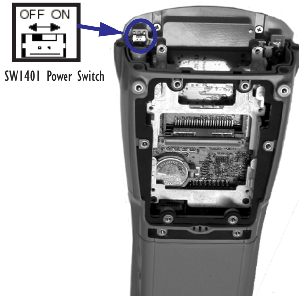
Figure 7.3 SW1401 Power Switch
