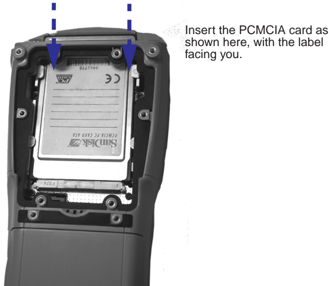
Figure 7.5 Inserting A PCMCIA Card
