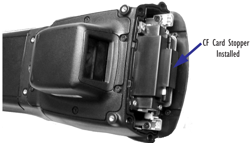
Figure 6.4 CF Stopper Installed
