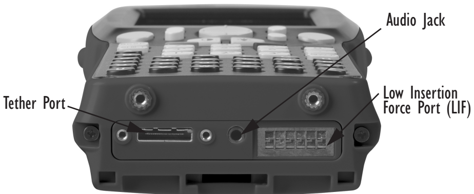
Figure 1.2 Tether Port, Low Insertion Force (LIF) Port And Audio Jack
