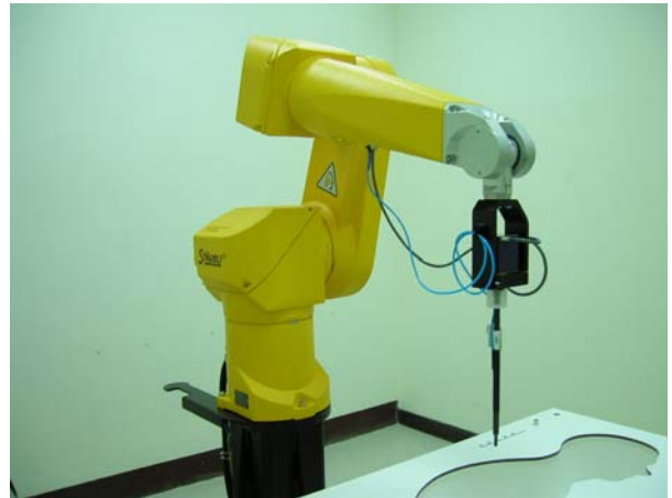
Fig. 5.2 Probe setup on robot
