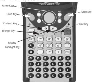
The keyboard is equipped with a set of standard keys along with a <ORANGE> and a <BLUE> modifier key to provide access to additional keys and system functions. These additional keys are colour coded in orange and blue print above the standard keys.
