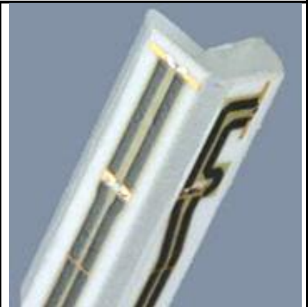
Fig 5.2 Photo of E-field Probe
