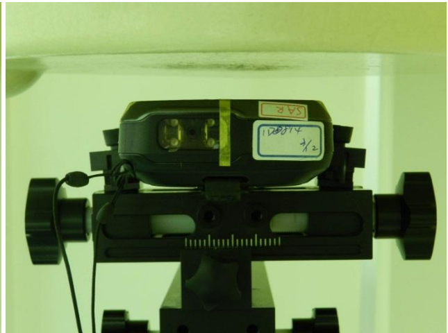
Front of the DUT with Phantom 1.5 cm Gap (DUT with Charger Snap Module 2)
