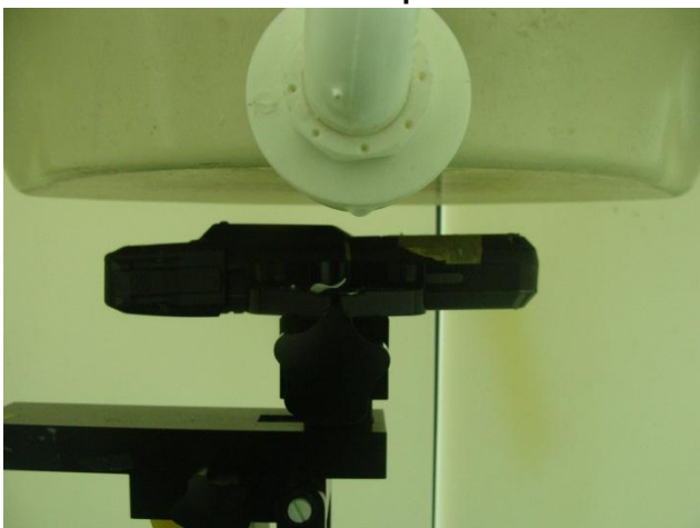
Rear Face of the DUT with Phantom 1.5 cm Gap (DUT with Charger Snap Module 1)
