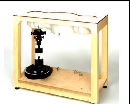
Fig 5.9 Photo of SAM Phantom
