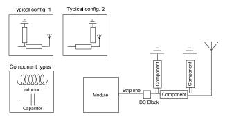
The matching network has to be individually designed using one, two or three components.
